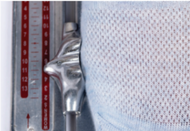
Heel to Ball (Arch Length): Position heel to ball device snug against the first metatarsal head. Record the arch length. As pictured, the measurement for the left foot is 11
