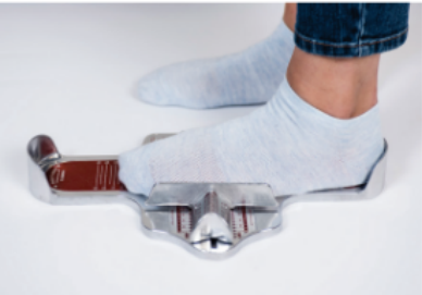
Place patient's heel at rear edge of the appropriate(right or left) heel cup
